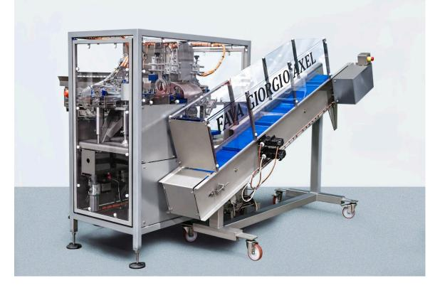
TDSAL automatic machine for clip removing and / or cutting in half, 45° or 90° angle, for cooked and cured products.
