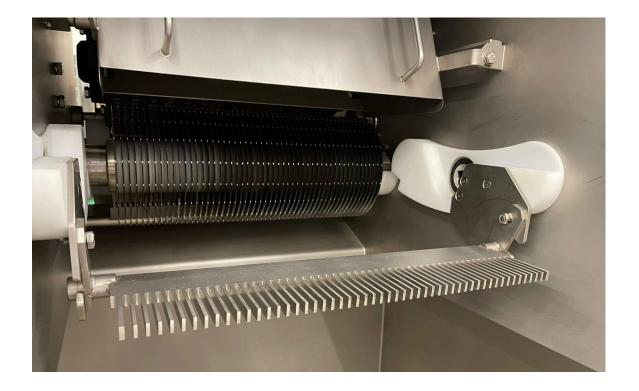
The **carve macerator** makes the deep cut of the meat on opposite parts following parallel directions, enormously increasing the absorption surface of brine and additives and favoring the meat proteins extraction.
