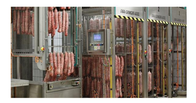
The **TFRC** system is the best solution to load and unload products on racks, trolleys or trees. It can load and unload **very high** trees, trolleys, racks and frames, **up to 5.8 meters** of height, handled by AGVs/LGVs or by overhead rail system. During the unloading phase it's also possible to unload one smoking stick at a time in order to feed the packaging or peeling lines.
