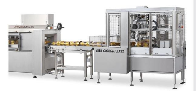
Our extremely **compact CONFSV vacuum bagging and packaging lines** can use either aluminum bags, shrink bags or taped bags. Easy adjustments ensure **excellent qualitative and quantitative results** and the different models can produce **from 360 to 720 pieces/hour**.
