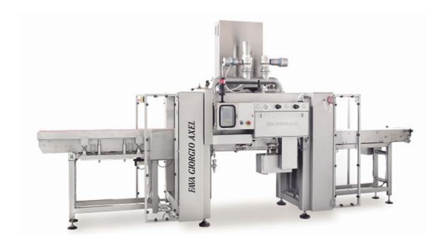
The structural typology of the **DCD vacuum thermosealing tunnel** allows easy insertion in production lines of products intended for cooking that use **both traditional** (deaeration) **and vacuum cooking** (thermosealed bags) technologies, in any case without renouncing the easy molding of products, whether anatomical or reconstructed.
