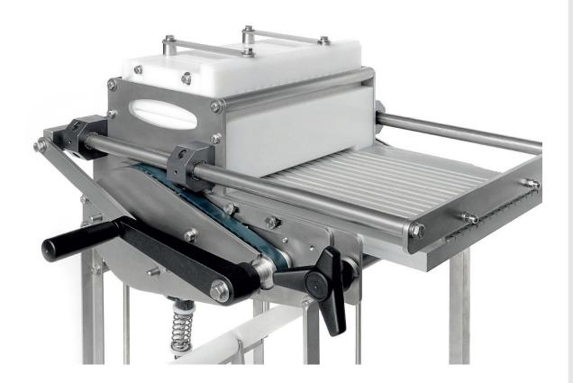
The **skewering machine for small kebab** inserts wood sticks (birch or similar) in meat to obtain **regular shape** skewers having a section from 15 x 15 mm till 37 x 37 mm, depending on the model (**standard or universal**).
